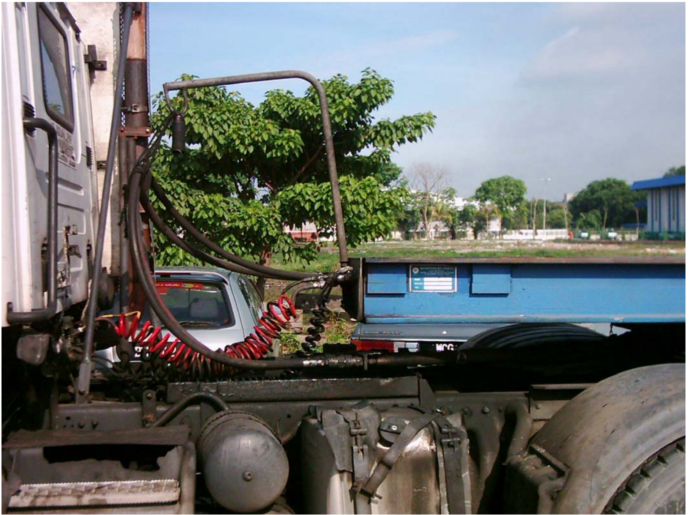
Figure 3: Photo showing looping of Hydraulic hoses to quick releases.
