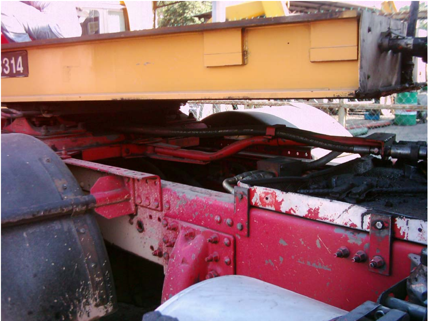
Figure 4: Photo showing Hydraulic hose swing arm.
